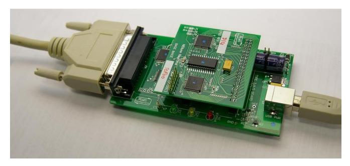
1. Before fitting NIStune board to programmer, fit "PGM" solder link. Ensure that no other links are fitted.
