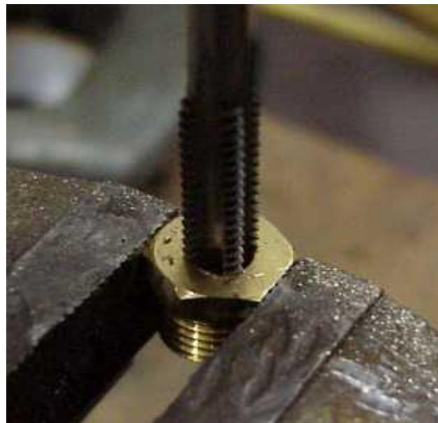
**4.** Take the jam nut and thread it part way up the Bolt. Wrap the Bolt with Teflon tape, to prevent air leaking between the threads, and thread the Bolt and nut into the Cap, place aside for now. I will refer to this as the 'Cap Assembly'.
