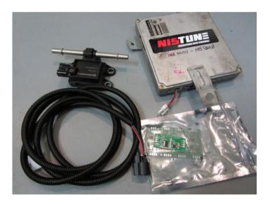
Requires multiple tunes (base tune on 98 octane, high end tune on E85 and then mix tune)
