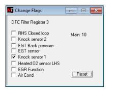
Turning this filter off will remove the DTC code and potentially also the Check Engine Light. However it will not stop further knock failure operations including timing retard. To disable knock retard, then following needs to be performed:
