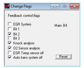
Disabling 'Knock Analysis' in the feedback flags will prevent any checking of the knock sensor connectivity. Turning off this flag will also result in access to normal fuel and timing maps without needing to 'stub' out the knock sensor lines on SR20 engines.
