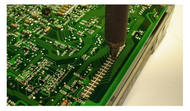
Tip: Be careful here. Don't attempt this unless you have the right equipment. It's quite easy to damage the board. Don't overheat the pads (about a second per pad is a safe maximum) or damage can easily result. If in doubt get somebody with the right equipment to do it for you. It's a 5 minute job so it shouldn't cost much.
