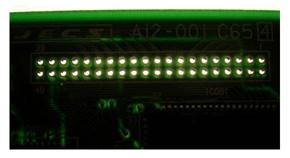
Hold the ECU up to the light and check that all the holes are clear. If any holes still have solder in them do not try to clear them out using a drill bit! The boards are multi-layer and it is quite likely that an internal connection will be damaged.
