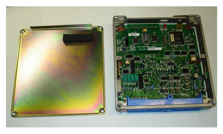
Remove the self adhesive backing from the foam rubber strip and fit it to the lid so that the board will be held firmly in position once the lid is fitted. This is best done by sitting the rubber strip (sticky side up) on top of the Simtek chip which is in the middle of the board, and then carefully fitting the lid.
