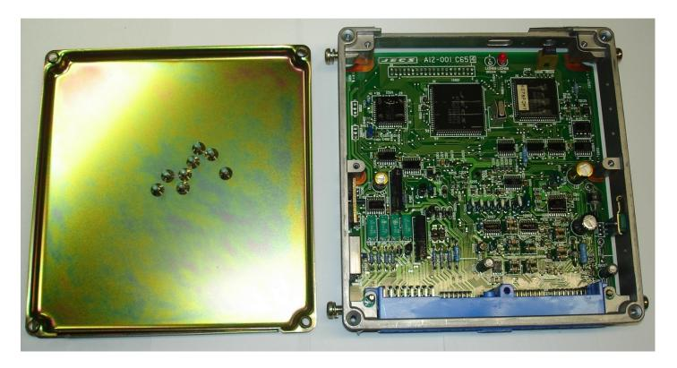
Tip: The screws that secure the covers will have thread locking compound applied from factory. This stuff really hangs on so make sure you use a driver with a tip which fits the screw head properly. We use a cordless drill. This may seem somewhat excessive but the combination of quality screwdriver tips available and being able to use an adjustable clutch makes for a very effective tool.
