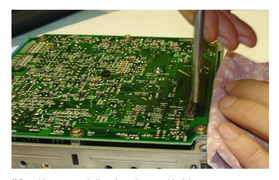
Clean off flux with acetone or similar solvent. Inspect solder joints.
