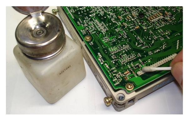
Using solvent or contact cleaner remove the coating around the 20+20 header area on both sides of the board and around the SMD jumpers (see later in document for photos).
