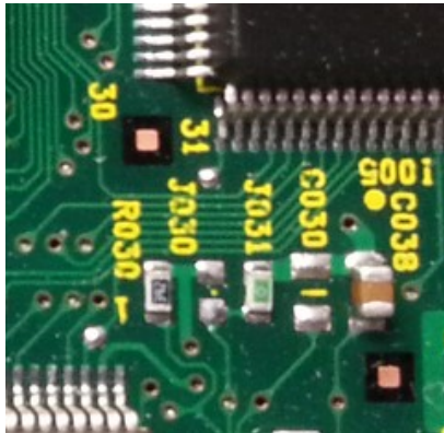
J031 to J030 – for A32 VQ30DE 1995 model: Top side of ECU between two small square chips
