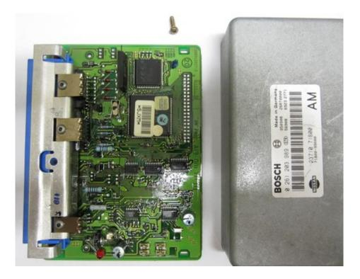
Once the rear cover is removed, unscrew the top screw to remove the top cover.
