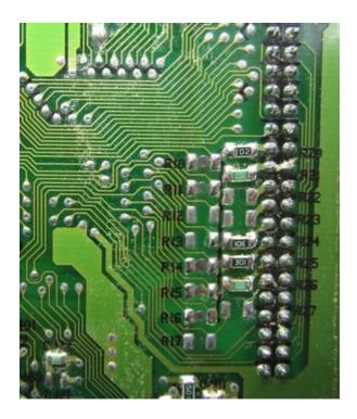
Note that the Type 5 board requires all resistor positions R1-R8 on the board to be connected using solder (blob each position)
