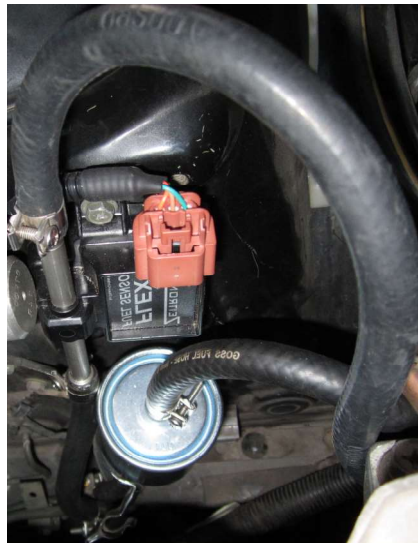
Image: Flex fuel sensor connected to fuel return line on S14 200SX
