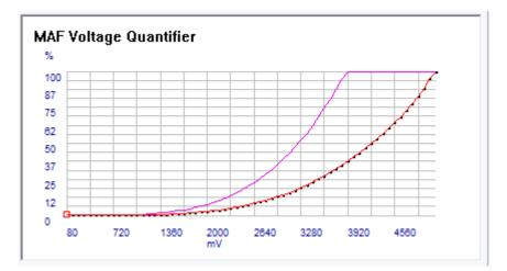
RED = normal VQ map for 3" HPXN1 sensor PURPLE = normalised VQ map for S14 SR20DET running 200rwkw with 3" HPXN1 sensor
