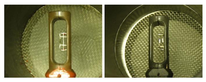
3. The genuine unit (left) has orange coating at the base of the MAF and a single dark coloured bead in the centre with a second ceramic strip sensor. The fake unit has white components and black plastic sensor mount.
