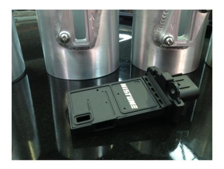
Slot style sensors may be used in larger tube sizes to increase maximum MAF range. When this is done (or the load measuring range of the sensor is more than required for the vehicle), then custom VQ maps are required. They are also more resistant to reversion having out flow vents on the sides of the sensor.
