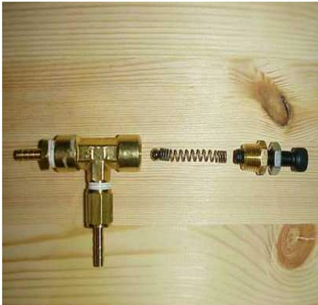
**6.1** Here is a basic cutaway view of what the internals will look like once the controller is completely assembled. Because the spring is sized closely to the inside of the Body, there is no need to modify the Body or spring to eliminate any lateral deflection that might occur if the clearance between the two components been greater.
