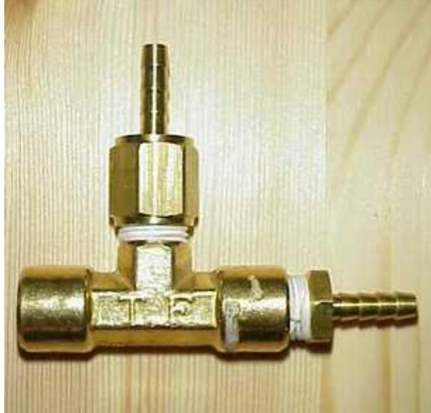
**6.** Place the ball bearing into the tee, so that it is now sitting at the bottom against the Base. Gently follow with placing the spring down on top of the bearing. Now take the Cap assembly and using some teflon tape thread it into the tee.
