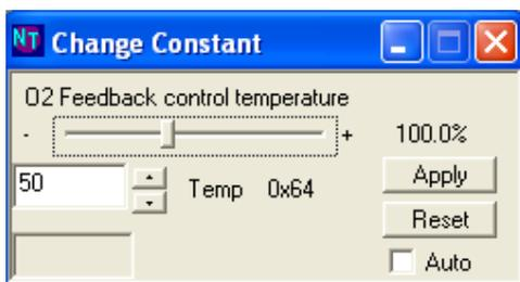
Or turning O2 sensor off in the feedback control flags
