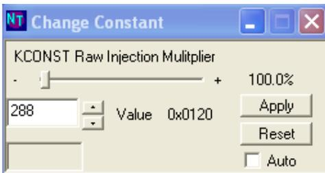
And then we add the Injection latency (sometimes known as pre ignition or void time). This is the opening / closing lag time of the injector. Bigger injectors need more latency to compensate for the increased opening / closing time. This will increase the Injector Time seen on the gauge by the amount entered in this box.
