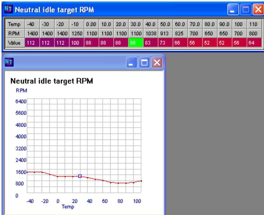
The ECU will then adjust the timing to attempt to reach the desired RPM. This is the main thing which stops the car from stalling, and timing will be increased when RPMs start dropping below the values in this table. Noticeably as the engine is colder, the target idle RPM is higher.
