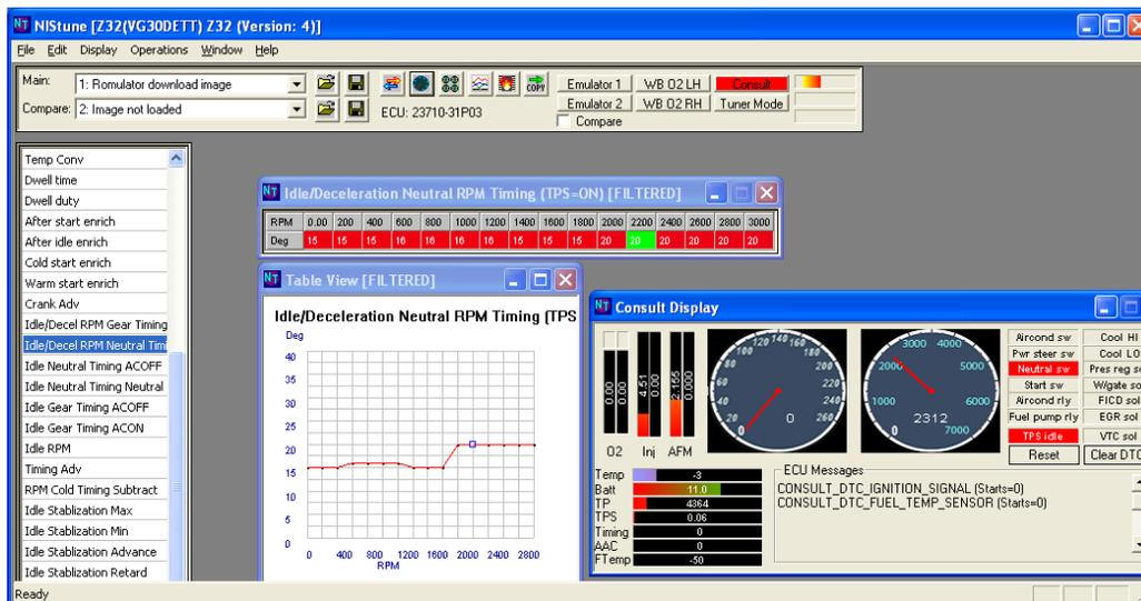
Idle / Deceleration RPM appear to be trigger points where for a particular RPM reached, if the timing is below the value in the chart then timing is cut to 0 until it recovers. Used to cut timing during deceleration.
