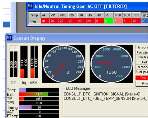
The timing is used as a combination of the various timing maps in the ECU and is pulled in depending on the temperature, TPS switch, neutral switch, TP and RPM conditions met in the ECU
