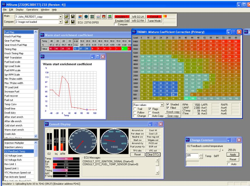
Check injection pulse width increases to 4.72ms (change due to alterations in fuel map)
