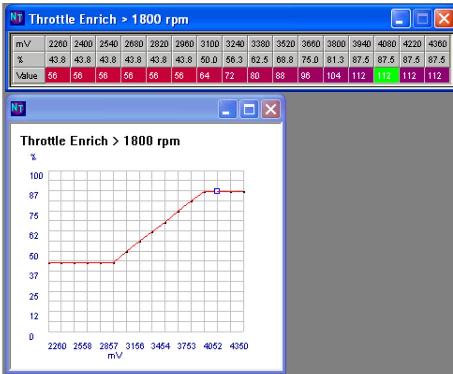
Once the engine is running, if the TPS idle switch is OFF then **TPS idle** will be highlighted in consult gauges and different tables are used. This is one of the tables used for enrichment coefficient based on vehicle RPM
