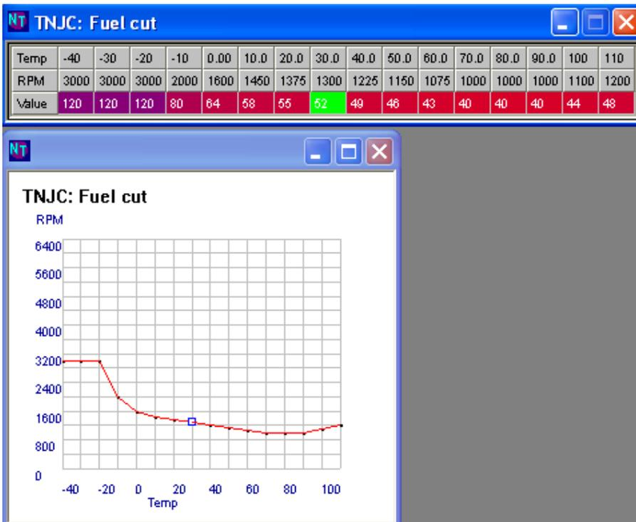
Here the fuel cut at normal operating temperature (85degC) will occur at 1000rpm
