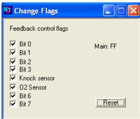
You can also use the 'O' key to turn off O2 feedback in the fuel map but only where the AFR is richer than 14.7:1. Nissan ECUs cannot turn off O2 feedback in this map for leaner than 14.7:1 because the map does not have the required numeric resolution to do so
