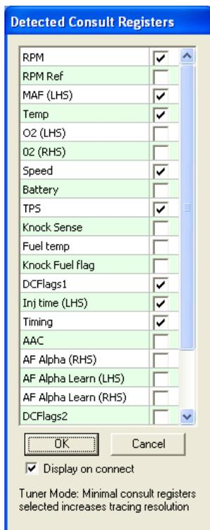
We require at least RPM, MAF, Temp, O2, Speed, TPS, DCFlags1, Injection Time and Timing to be recorded. If you are able to connect up a wideband unit, then you can also capture that in parallel with the log
