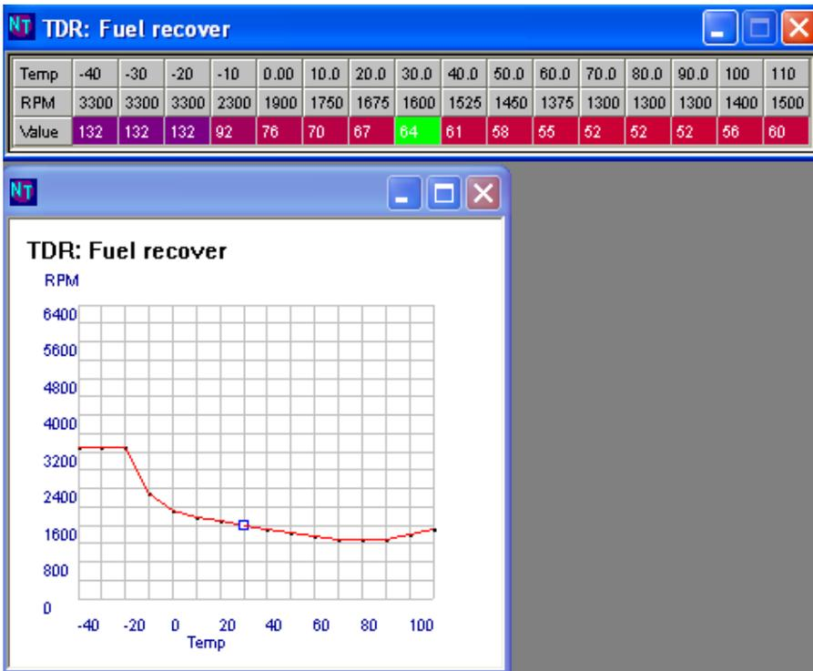
The fuel recovery will resume injection when the ECU has reached the desired RPM in this table (85degC will occur at 1300 rpm)
