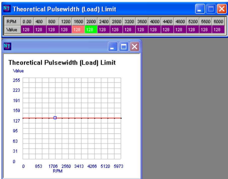
That gauge that you saw the TP value earlier, if it goes above the TP values in the above table for the given RPM then the ECU will perform a fuel cut. This is a protection mechanism provided by the Nissan ECU for when the engine over boosts due to problem with controlling the waste gate actuator.
