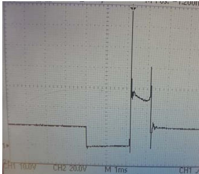
*Picture above: Output to primary coil from power transistor (triggered from ECU). Secondary coil output is what causes the massive spike and creates the spark*
