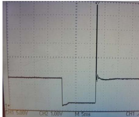
The main parameter for changing injector pulse width which will affect the vehicle regardless of current map(s) being accessed is the K constant (or injection multiplier)
