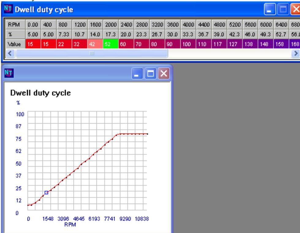
The remaining timing tables are used to determine when to fire the spark, relative to position of the cylinder. This is measured in BDTC. The engine must be at factory BDTC settings on the CAS for Nistune to accurately display the timing. The timing is what the ECU 'thinks' the engine is set to. If the CAS timing settings are wrong, then so will the Nistune displayed settings.
