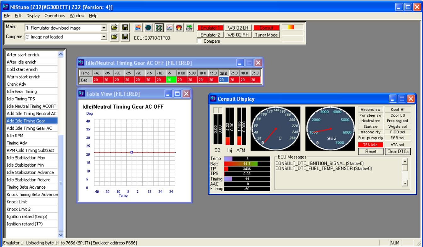
In the example below, altering the timing from 20 to 5 changes the timing from 35BDTC to 20BDTC
