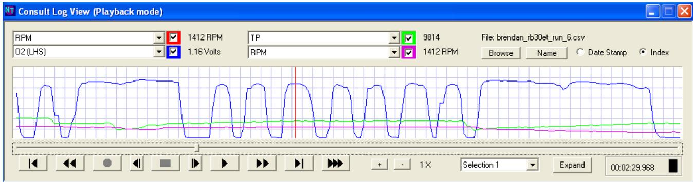
You will see from the run below that the O2 (LHS) on this RB30ET bounces above/below trigger voltages. We have the red line on 1.16 volts just as the ECU picks this up, it will lean the mixture.
