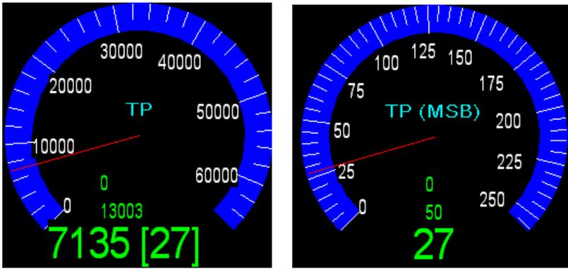
The main number is the TP number and the second number in brackets is the TP / 256. This is known as TP (MSB) in later versions of Nistune (where MSB = Most Significant Byte). The TP is basically a load indication of the ECU. It is used to index fuel and timing maps inside the ECU and the amount of incoming air through the airflow meter will determine where things are indexed.
